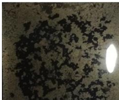
Figure 13 - Graphene agglomeration attains after the drop-casting method on a polished surface.
