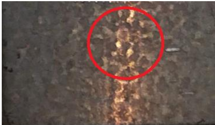
Figure 14 - GO coating defect exhibited on the polished surface created by spray deposition.
